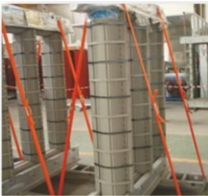
CRGO stacked assembled core
